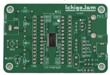
2. R1~R4 Resistor (no directions, cut back)
